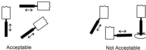
Figure 1 – Correct and Incorrect Angles of Measurement
