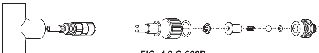
FIG. 4.9 C-600P INJECTION/CHECK VALVE TEE INSTALLATION AND EXPLODED VIEW
