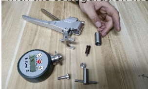
④ Take out the pressure cylinder and replace it with a new needle
