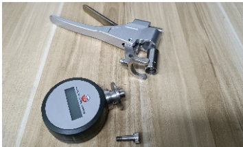
② Remove the pressure cylinder
