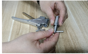
③ Twist the pressure cylinder with the configuration wrench
