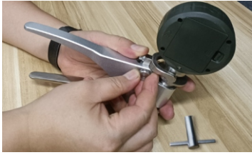
① Unscrew the handle nut
