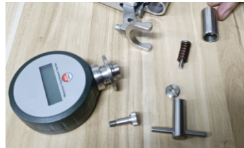
④ Take out the pressure needle and replace it with a new needle
